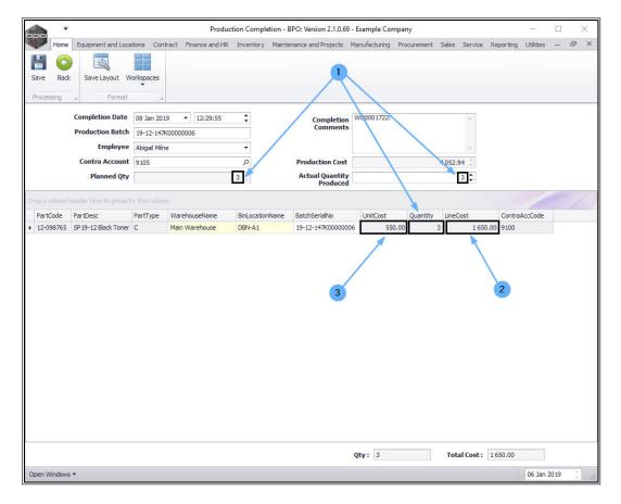
In this example the Actual Quantity Produced has been increased to 4.
